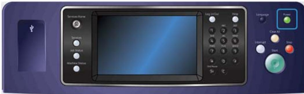
1. Press the **Power** button on the control panel.
